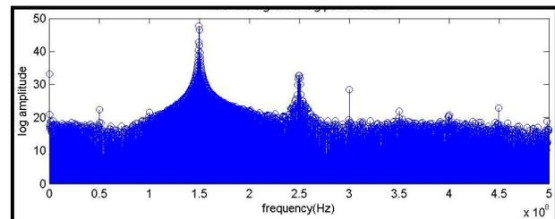
Fig 9 MATLAB FFT output for CW over Pulse case
