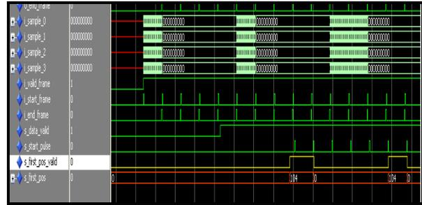
Fig. 3. Peak Detector module output for 800 MHz 100 ns Pulse
