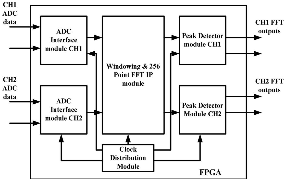
Fig. 2: FPGA Based Signal Processing architecture
