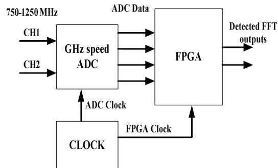
Fig.1: Pulse Detection Architecture for Digital ESM Receiver
