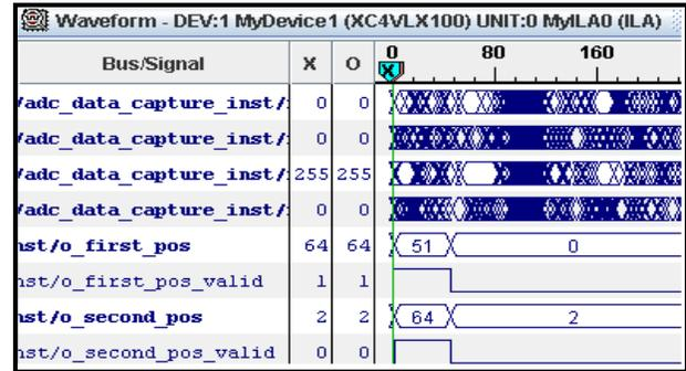
Fig 6 Xilinx Chipscope Pro output Pulse over Pulse signal case
