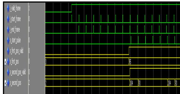
Fig. 4. Peak Detector output for 800 MHz 100 ns Pulse overlapped with 850 MHz CW case
