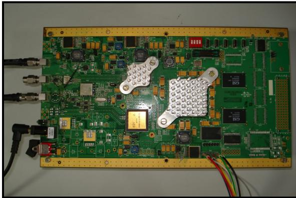
Fig.5 Digital Receiver Hardware
