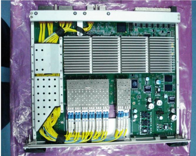
Fig. 4: IDBF card with optical cables routed. Ready to be put into mechanical enclosure. Heat sinks cover the FPGAs.
