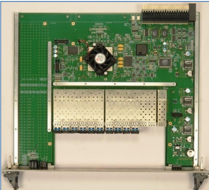
Fig. 5: FDBF card without optical cables. FPGA is mounted with active heat sink for lab testing
