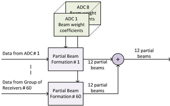
Fig. 2: Partial Beam Formation in DBF
