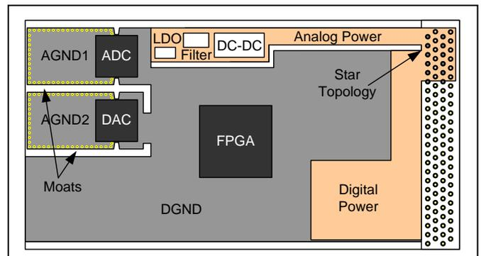
Figure 6: Isolation between Digital and Analog Supply
