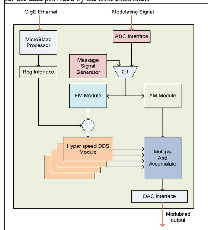
Figure 2: Baseband Generator RTL Block Diagram
