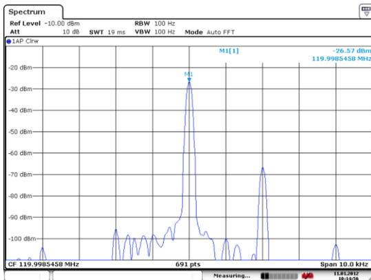
SSB Modulation with 35dB Carrier Suppression
