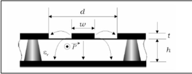
Figure 4: CPWG Cross-Section
